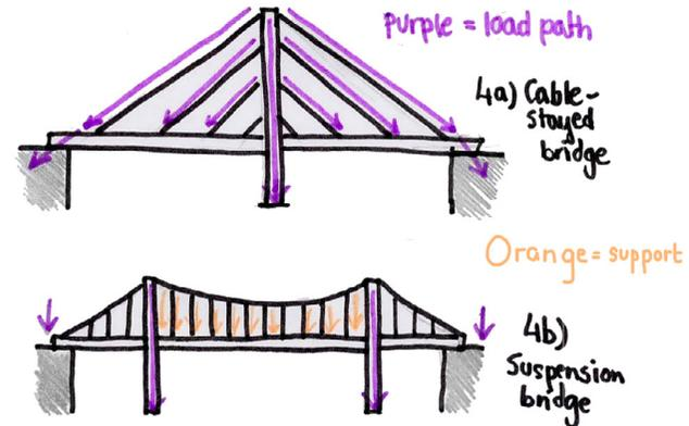
The towers support the majority of the weight as compression pushes down on the suspension bridge's deck and then travels up the cables, ropes or chains to transfer compression to the towers. The towers then dissipate the compression directly into the earth.
